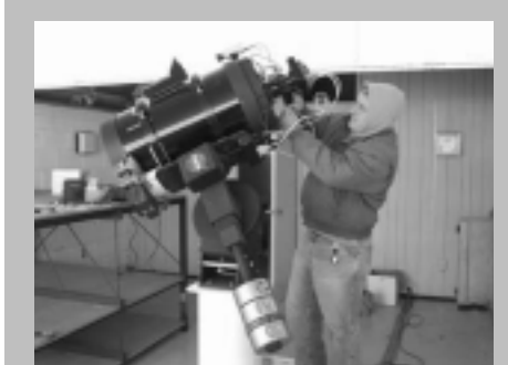
Mark Leon, Code D, working on the remote control and communications of the 14-inch telescope.
