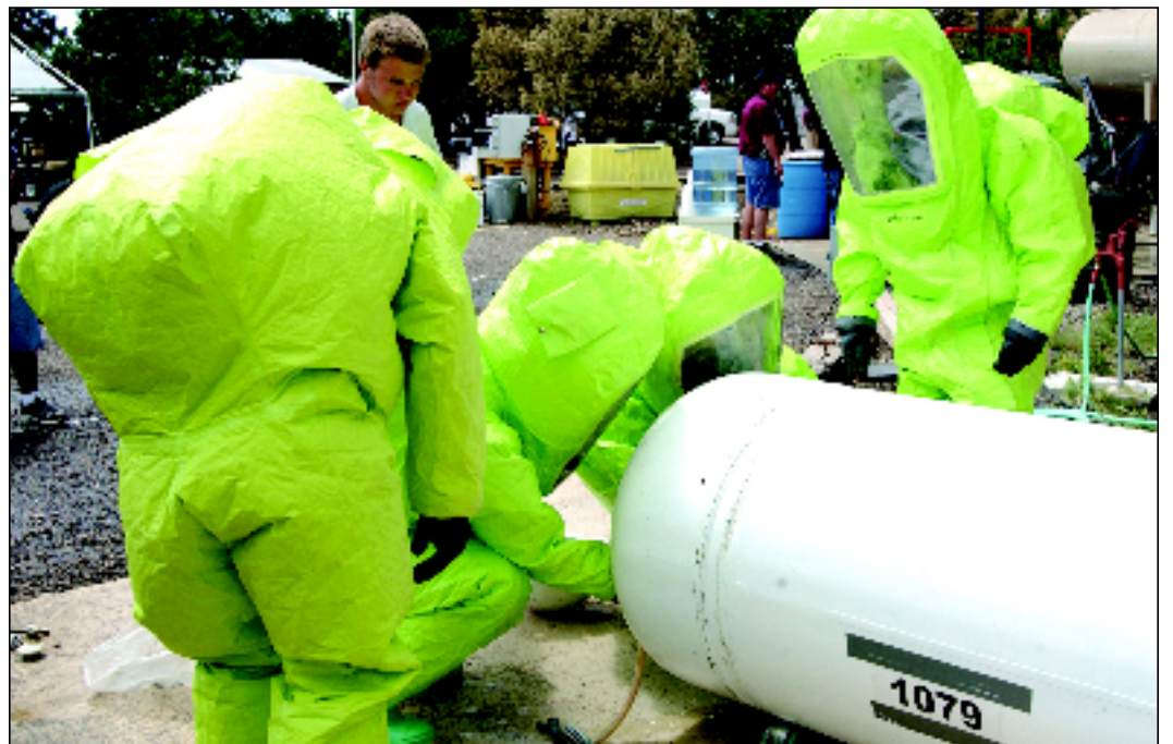
The Los Alamos National Laboratory team, decked out in their fully encapsulated Class A protective equipment, tackle a simulated one-ton leaking compressed gas/chlorine tank. Chlorine and compressed gas leaks can be very complicated problems, made even more difficult by the Class A protective suits that limit the responder's vision and communications.
