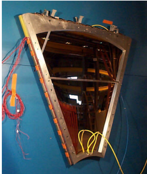
Figure 16: A photograph of a MuTr station-2 octant. A cathode plane is made of etched 25- \mu\text{m} copper coated mylar foils.
