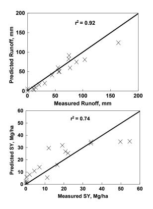
Figure 2. Relationships between predicted runoff and sediment yields (SY) from the WEPP Watershed model and measured values for a 17-year period (1975-1991).
