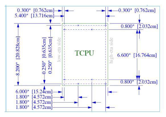
Clearance from top of TCPU to underside surface of cover assembly = 0.629 inches.
