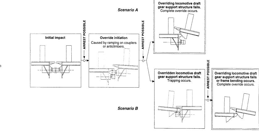
Figure 2. Two Potential Head-On Collision Override Scenarios
