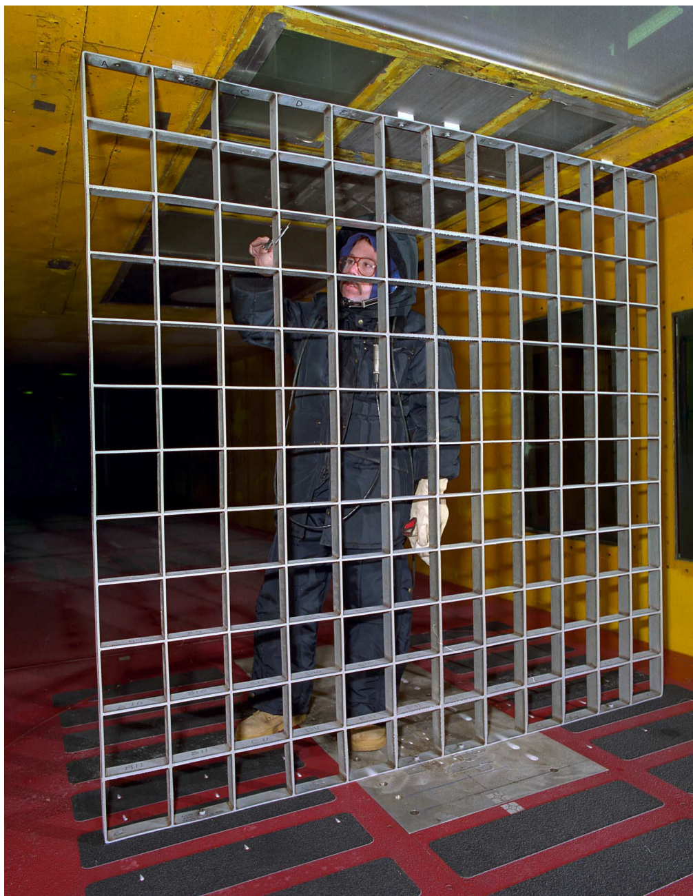
Figure 2.—The icing grid used for cloud uniformity measurement.
