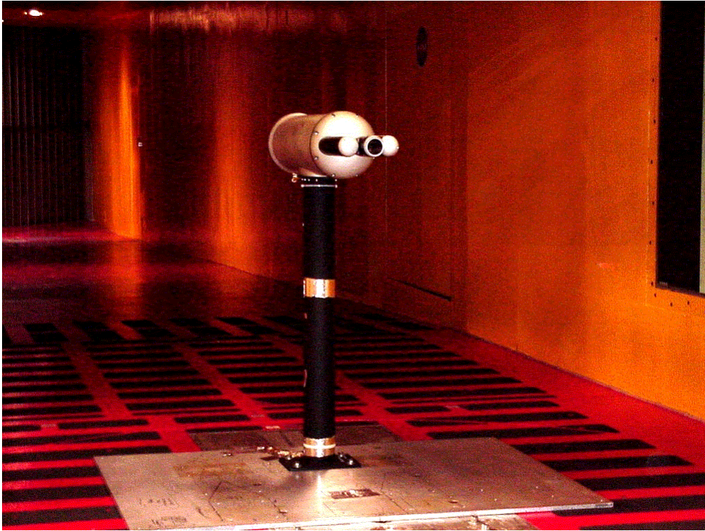
Figure 9.—Picture of the FSSP droplet sizing instrument mounted in the test section of the IRT.
