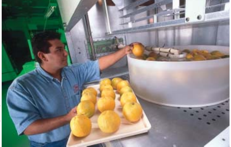
Technician Carlos Solis, of the ARS Kika de la Garza Subtropical Agricultural Research Center, in Weslaco, Texas, places oranges in a water bath heated with radio waves to kill fruit flies. The water is circulated to heat the oranges uniformly and prevent fruit damage.
