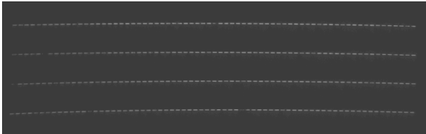
Fig. 4. Nearfield image of the laser diode array under normal operation. Each bright dash is one emitter. This device has four rows of emitters.
