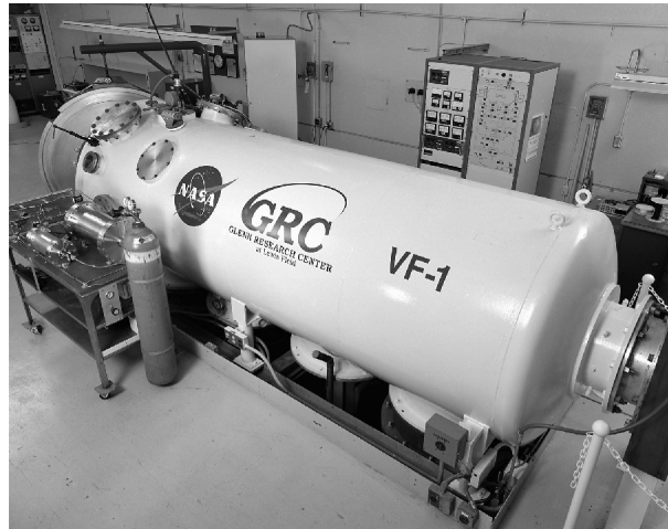
Figure 5. VF-1 vacuum chamber and propellant plenum test cart.
