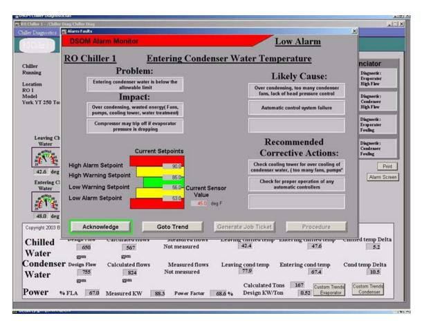
Figure 2: Chiller Diagnostician Alarm Display
