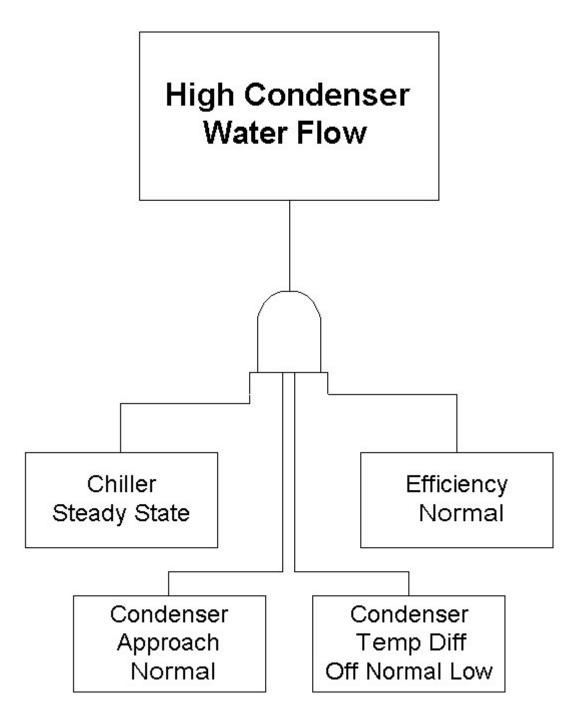
Figure 4: Logic block diagram for High Condenser Water Flow
