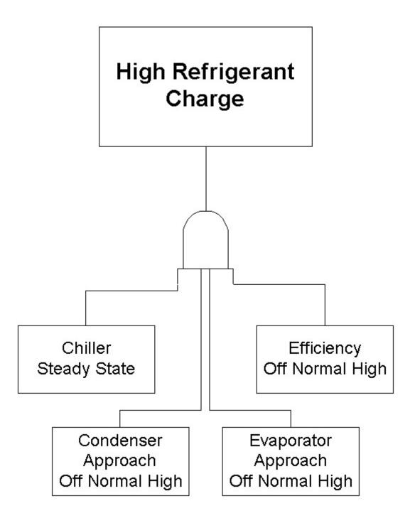
Figure 6: Logic Diagram for High Refrigerant Charge Diagnostic
