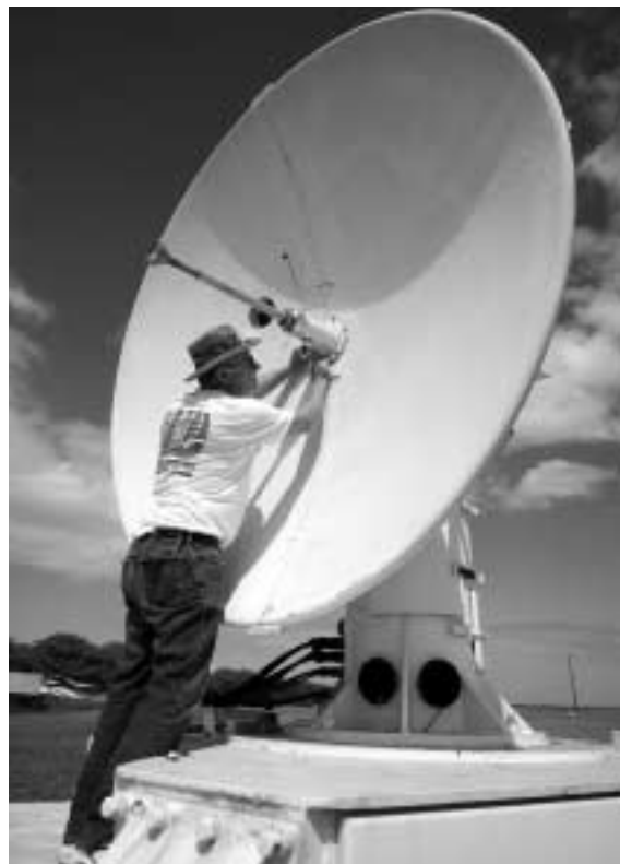
ANDY JONES (2333) installs a motor assembly on a tracking radar in preparation for a balloon launch.
