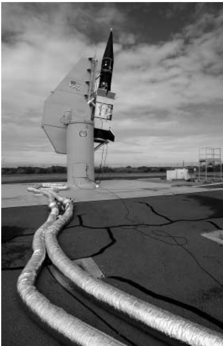
FM-5 TARGET ROCKET on Pad 1's rail launcher ready for liftoff. The flexible conduit supplies cold air to a fall-away cooling chamber affixed to the rocket, which keeps critical electronics cool until launch.
