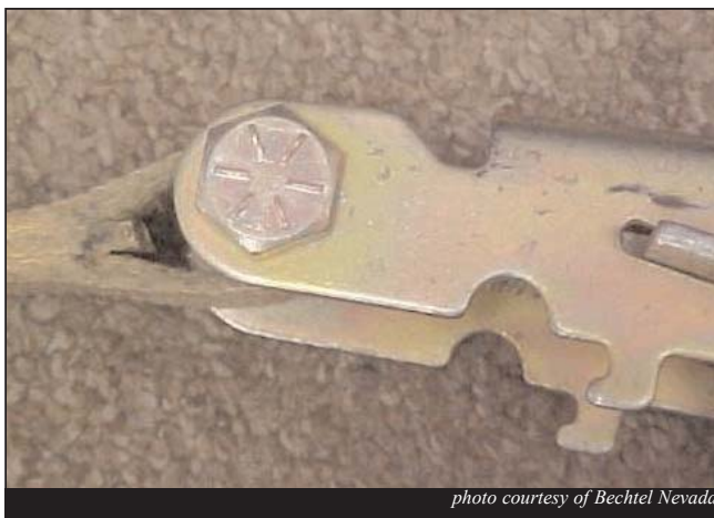
An example of a counterfeit bolt found on a ratchet assembly at the NTS.
