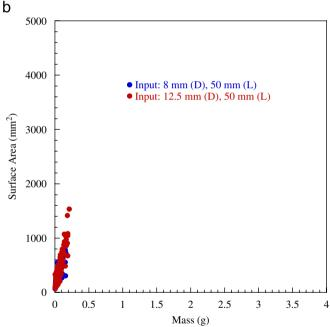
Fig. 8. (a) Calculated surface area plotted as a function of mass for firebrands produced from burning trees. (b) Calculated surface area plotted as a function of mass for firebrands produced from the firebrand generator.
