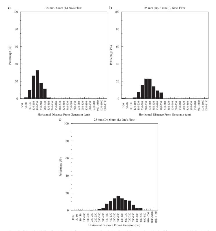
Fig. 6. Evolution of the firebrand spatial distribution as a function of applied wind speed. Data are shown for the disk geometry only: (a) 3 m/s wind speed, (b) 6 m/s wind speed and (c) 9 m/s wind speed.
