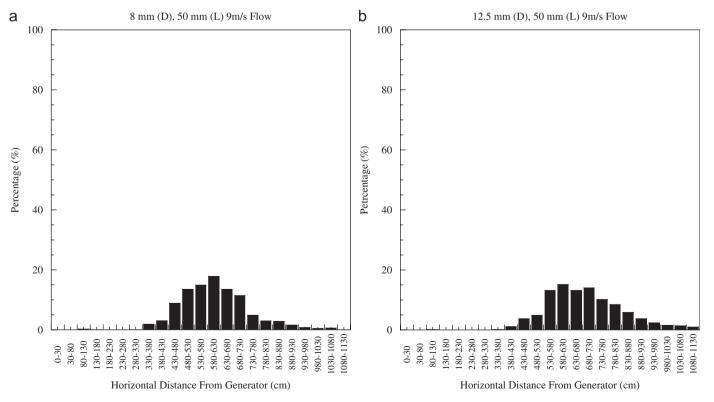
Fig. 7. Firebrand spatial distribution at 9 m/s: (a) 8 mm diameter, 50 mm long cylinders and (b) 12.5 mm diameter, 50 mm long cylinders.
