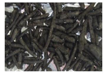
Fig. 3. Digital photograph showing typical firebrands collected when 8 mm diameter,  $50\,\mathrm{mm}$  long cylinders were used.
