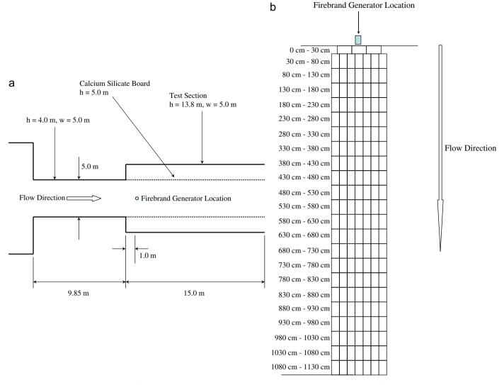
Fig. 2. (a) Schematic of the FRWTF. (b) Layout of pans used to collect the firebrands produced from the generator.
