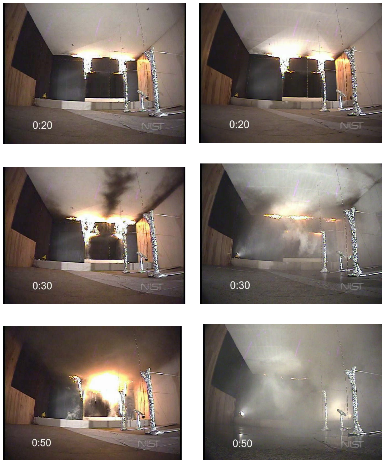
Figure 4-20. Still frames taken from video of full-scale mock-up experiments. Time after ignition is indicated in lower left of each frame. Left column: unsprinklered; right column: sprinklered (first head activates at 24 seconds)
