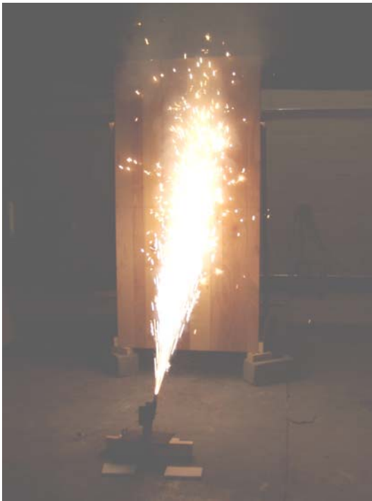
Figure 4-14a. Gerb impinging on wood panel
