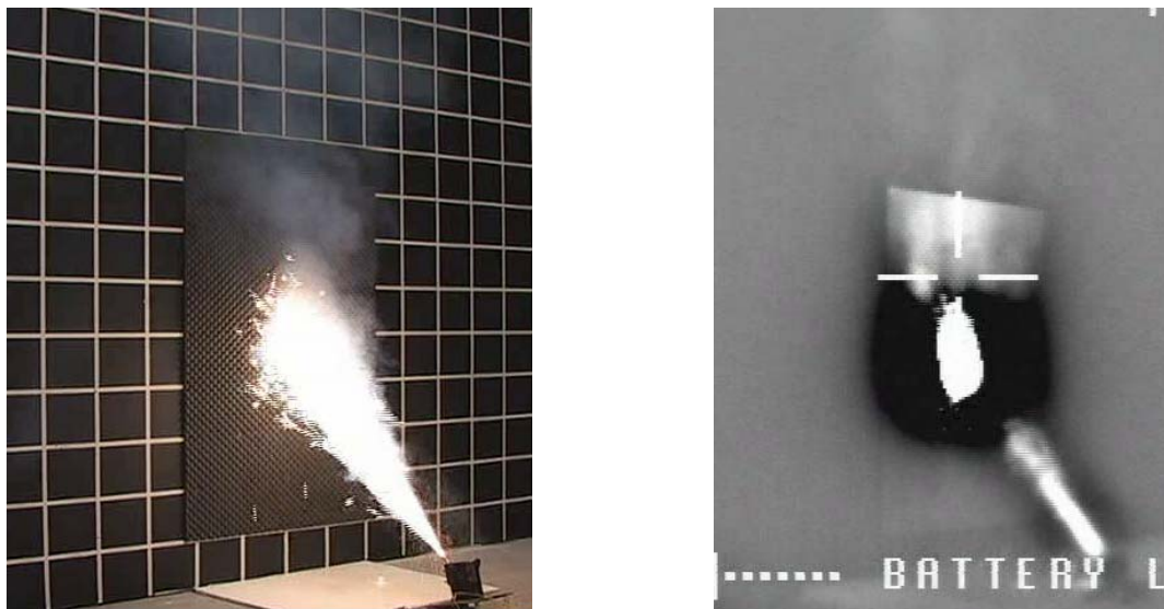
Figure 4-13f. Standard and Infrared Video Images of Gerb Discharge onto a Non-fire Retarded Polyurethane Foam Sheet on Gypsum Board Wall at t = 10 seconds.
