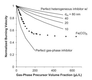
Fig. 27. Calculated normalized burning velocity for several diameters  $d_{\rm m}$  of ideal heterogeneous inhibitor. Also shown are Fe(CO)<sub>5</sub> data and calculated normalized burning velocity using the perfect gas-phase inhibitor mechanism [41].
