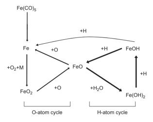
Fig. 12. Schematic diagram of radical recombination reaction pathways is found to be important for  $CO/H_2/O_2/N_2$  flames. Thicker arrows correspond to higher reaction flux. Reaction partners are listed next to each arrow [74].
