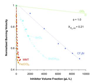
Fig. 16. Normalized burning velocity of premixed  $CH_4/O_2/N_2$  flames inhibited by  $CO_2$ ,  $CF_3Br$ ,  $Sn(CH_3)_4$ ,  $SnCl_4$  [49], MMT, and  $Fe(CO)_5$  ( $T_{in} = 353 \text{ K}$  for all data except  $Sn(CH_3)_4$  and  $SnCl_4$  which are at 298 K) (points: experiments; lines: curve fits) [10].
