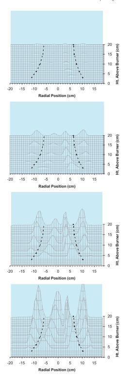
Fig. 35. Scattering cross section for laser light at 488 nm as a function of radial position and height above burner in methane–air cup-burner flame with 8% CO<sub>2</sub> and Fe(CO)<sub>5</sub> in air at specified volume fraction. Dotted lines show flame location from a digitized video image of the uninhibited flame [115]. Top to bottom frames have (100, 200, 325, and 450)  $\mu L/L$  of Fe(CO)<sub>5</sub>, respectively.
