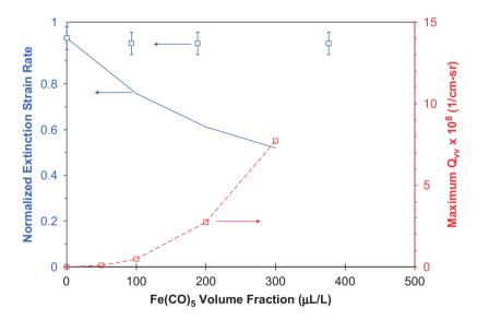
Fig. 33. Effect of Fe(CO)<sub>5</sub> added to the air stream of a diluted methane–air counterflow diffusion flame. The experimentally measured (points) and numerically calculated (solid line) normalized extinction strain rate [43] are shown (left axis) as a function of Fe(CO)<sub>5</sub> volume fraction in the air stream. The maximum scattering cross section (right axis), obtained from the results in Fig. 30 is also shown for increasing  $X_{\text{inh}}$  [50].
