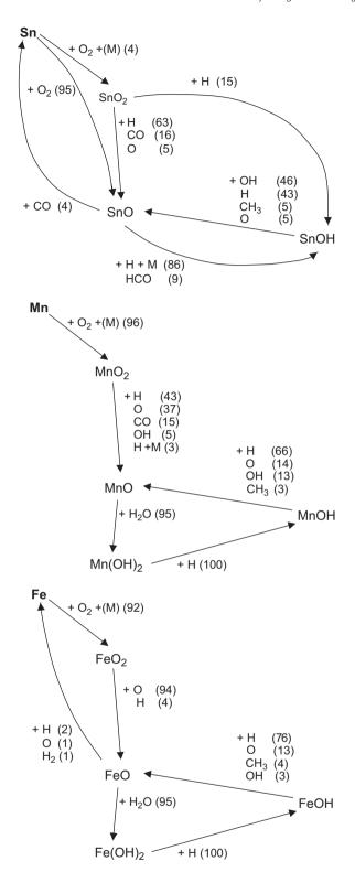
Fig. 19. Reaction pathways for Sn, Mn, and Fe in a premixed methane–air flame ( $\phi = 1.0$ ,  $X_{\rm O_2,ox} = 0.21$ ,  $T_{\rm in} = 353$  K). TMT, MMT, and Fe(CO)<sub>5</sub> present at (1963, 128, or 105)  $\mu$ L/L, respectively. The numbers in parentheses are the fractional consumption (percent) of the reactant molecule.
