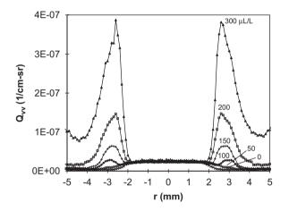
Fig. 23. Measured scattering cross section through a stoichiometric  $CH_4$ -air flame 7 mm above the burner rim at various inhibitor volume fractions [41].
