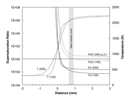
Fig. 15. Temperature and supersaturation ratio of Fe and FeO as a function of position through a premixed  $CH_4$ -air flame with  $Fe(CO)_5$  added at 100 or  $500 \,\mu L/L$  [9].
