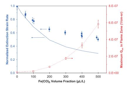
Fig. 29. Correlation between inhibition effect and maximum  $Q_{vv}$ . Filled points are experimental normalized  $a_{ext}$ , solid line is calculated  $a_{ext}$  [43]. Open symbols connected by dotted lines are maximum measured  $Q_{vv}$ . Particle data collected at 75% of  $a_{ext}$  [45].
