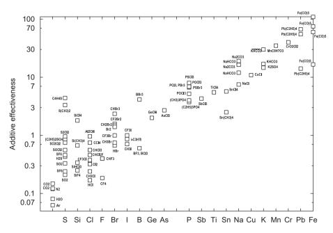
Fig. 2. Relative inhibitor effectiveness. Additive effectiveness is presented in coefficients of efficiency relative to CF<sub>3</sub>Br. The compounds considered are mostly liquids or solids [78].
