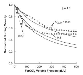
Fig. 3. Normalized burning velocity of premixed  $CH_4$ -air flames with added  $Fe(CO)_5$  at varying  $X_{O_2,ox}$  (points: experimental data; lines: 1-D numerical predictions with gas-phase inhibition chemistry) [9].
