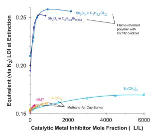
Fig. 41. Equivalent  $N_2/O_2$  limiting oxygen index for extinction of polyethylene (PE) halogen blends or methane–air cup burner flames with MMT, Fe(CO)<sub>5</sub>, and Sn(CH<sub>3</sub>)<sub>4</sub> [152].
