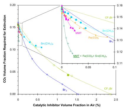
Fig. 34. Volume fraction of  $CO_2$  required for extinction ( $X_{CO_2,ext}$ ) of methane–air cup burner flames as a function of the volume fraction of catalytic inhibitor added to the air stream. Inset shows region in dotted box with expanded scales (points: experiments; lines: curve fits) [115].
