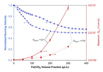
Fig. 24. Normalized burning velocity [9] and maximum  $Q_{vv}$  for  $\phi = 1.0$  CH<sub>4</sub> flame with  $X_{O_{v},ox} = 0.21$  and 0.24 [41].
