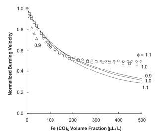
Fig. 4. Normalized burning velocity of premixed CH<sub>4</sub>–air flames with added Fe(CO)<sub>5</sub> at varying  $\phi$  (points: experimental data; lines: 1-D numerical predictions with gas-phase inhibition chemistry) [9].
