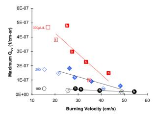
Fig. 26. Maximum  $Q_{vv}$  for flames of CH<sub>4</sub> (open symbols) and CO (closed symbols) as a function of the burning velocity. The letters correspond to the adiabatic flame temperature (low, medium, and high: 2220, 2350, and 2470 K), while the symbol shape (square, diamond, and circle) corresponds to the loading of Fe(CO)<sub>5</sub>: (100, 200, and 300)  $\mu$ L/L [41].
