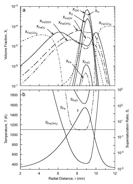
Fig. 39. (a) Calculated volume fraction  $X_i$  for iron-containing and major species as a function of radial position at the height above the burner of 4.8 mm (corresponding to the location of the reaction kernel in the flame base) and (b) the super-saturation ratio,  $S_i$ , for Fe, FeO, and Fe(OH)<sub>2</sub> [115].
