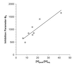
Fig. 5. Variation of inhibition parameter  $\Phi_0$  [124] with degree of H-atom super equilibrium in premixed methane—air flames with added Fe(CO)<sub>5</sub> (line: linear curve fit) [9].
