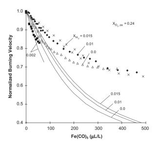
Fig. 10. Normalized burning velocity for  $CO/O_2/H_2/N_2$  flames with added  $Fe(CO)_5$  with  $X_{O_2,ox} = 0.24$  and varying  $X_{H_2}$  (points: experiments; lines, numerical calculations) [74].
