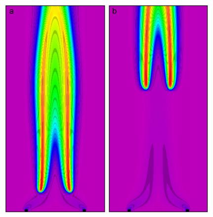
Fig. 37. 2-D color map of calculated temperature in cup-burner methane—air flames with 10% CO<sub>2</sub> in the oxidizer stream, and (a) 0.011% and (b) 0.012% Fe(CO)<sub>5</sub> volume fraction in the air stream, illustrating the blowoff phenomenon [115].
