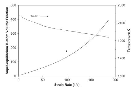
Fig. 8. Super-equilibrium ratio and temperature variation with strain for counterflow CH<sub>4</sub>-air flames [151].
