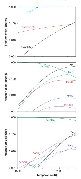
Fig. 20. Fraction of Sn-, Mn-, and Fe-species at equilibrium in methane-air flames as a function of temperature.
