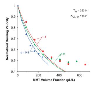
Fig. 18. Normalized burning velocity of premixed  $\text{CH}_4/\text{O}_2/\text{N}_2$  flames inhibited by MMT with  $X_{\text{O}_2,\text{ox}} = 0.21$  and  $\phi = 0.9$ , 1.0, and 1.1 (points: experiments; lines: numerical calculations) [10].
