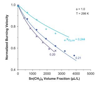
Fig. 17. Normalized burning velocity of premixed  $CH_4/O_2/N_2$  flames inhibited by TMT, with  $\phi = 1.0$  and  $X_{O_2,ox} = 0.20$ . 0.21, and 0.244 (points: experiments; lines: numerical calculations) [10].
