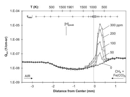
Fig. 30. Measured scattering profiles in  $CH_4$ -air counterflow diffusion flame with inhibitor in the fuel. The calculated temperature and point of peak H-atom mole fraction are marked on the upper x-axis, and the vertical line denotes the calculated location of the stagnation plane. Strain rate =  $330 \, \text{s}^{-1}$  [45].
