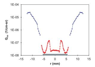
Fig. 22. Scattering cross section  $Q_{vv}$  as a function of the radial distance r from the burner centerline at 7 mm height in stoichiometric CH<sub>4</sub>–air flame with 200  $\mu$ L/L of Fe(CO)<sub>5</sub> [41].
