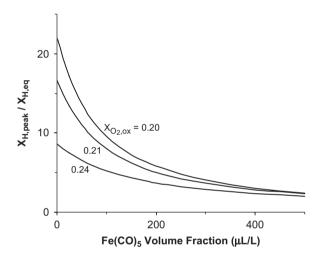
Fig. 14. Calculated ratio of peak and equilibrium values of [H] in premixed  $CH_4/O_2/N_2$  flames with added  $Fe(CO)_5$  at different  $X_{O_3,ox}$  [42].
