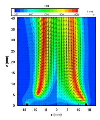
Fig. 36. Calculated temperature (color scale) and velocity vectors (arrows) for methane–air cup-burner flame with an oxidizer stream  $CO_2$  volume fraction of 10%, with (left) and without (right) an added Fe(CO)<sub>5</sub> volume fraction of  $100 \,\mu L/L$  [115].
