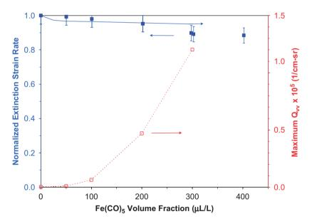
Fig. 31. Effect of Fe(CO)<sub>5</sub> added to the fuel stream of a methane–air counterflow diffusion flame. The experimentally measured and numerically calculated normalized extinction strain rate [43] are shown (left axis) as a function of Fe(CO)<sub>5</sub> volume fraction in the fuel stream. The maximum scattering cross section (right axis), obtained from the results in Fig. 30 is also shown for increasing  $X_{\text{inh}}$ .
