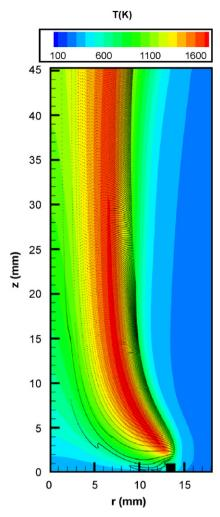
Fig. 40. Calculated particle trajectories for free-molecular-regime particles in a  $CH_4$ -air flame with 10%  $CO_2$  in the oxidizer stream [115].
