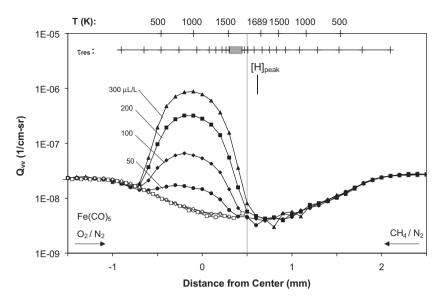
Fig. 32. Scattering profiles through a counterflow diffusion flame of 30%  $O_2/70\%$   $N_2$  and 80%  $CH_4/N_2$ . The calculated temperature and point of peak H-atom mole fraction are marked on the upper x-axis, and the vertical line denotes the calculated location of the stagnation plane. Fe(CO)<sub>5</sub> is added to the oxidizer stream at the indicate volume fraction. The estimated residence time for 5 nm particles is shown as 10 ms intervals in the hatched line near the top [45].
