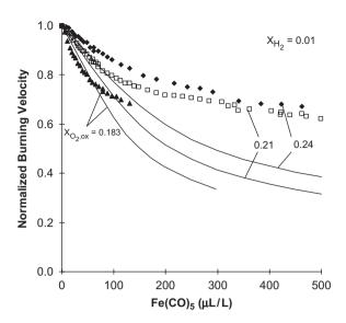
Fig. 9. Normalized burning velocity for  $CO/O_2/H_2/N_2$  flames with added  $Fe(CO)_5$  with  $X_{H_2} = 0.01$  and varying  $X_{O_2,ox}$  (points: experiments; lines: numerical calculations) [74].
