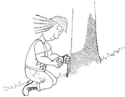
Figure TD-10. Measure char height on the downhill side of the tree.
