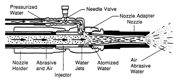
Figure 2-6. Nozzle for air abrasive wet blast.
