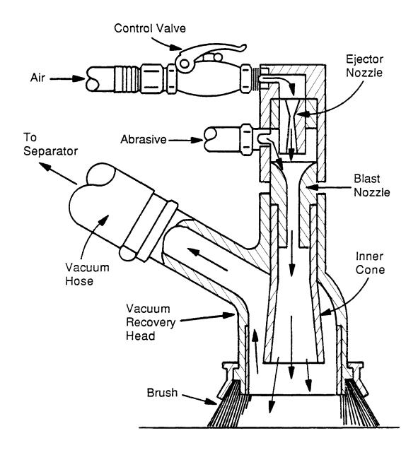
Figure 2-5. Schematic of vacuum blaster head.
