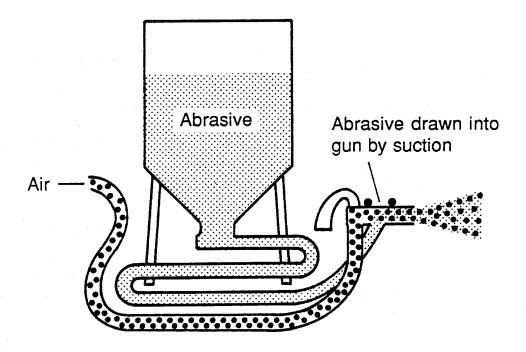
Figure 2-1b. Suction-tape blasting machine.
