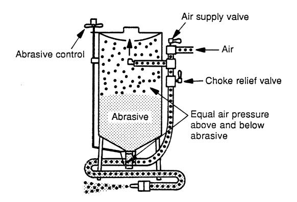
Figure 2-2. Pressure-type blasting machine.
