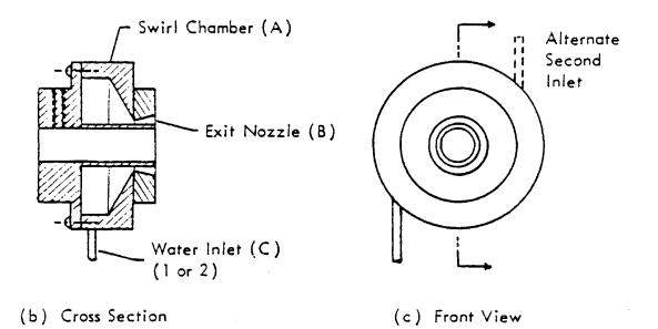
Figure 2-7. Water curtain device for abrasive blast nozzle.
