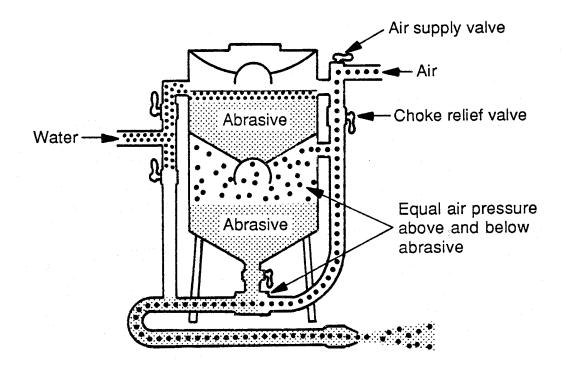
Figure 2-3a. Wet blasting machine.
