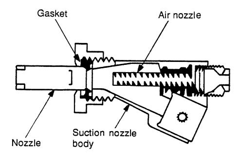
Figure 2-1a. Suction blast nozzle assembly.
