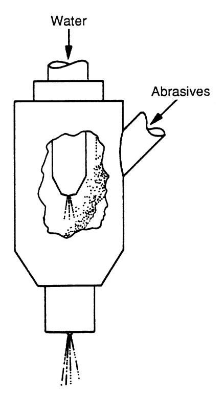
Figure 2-4. Hydraulic blasting nozzle.
