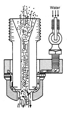
Figure 2-3b. Adapter nozzle converting a dry blasting unit to a wet blasting unit.
