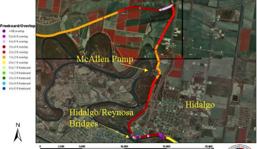
Levee reach, commonly referred to as the Hidalgo Loop levee, ties into the south levee of the Main Floodway and continues in a southerly direction for 3.3 miles to the Hidalgo/Reynosa bridges. Levee protects the city of Hidalgo from flooding. Levee is approximately 6 feet deficient in height throughout the reach, with only marginal structural integrity problems. Estimated Construction Cost - \$ 6.7 million
