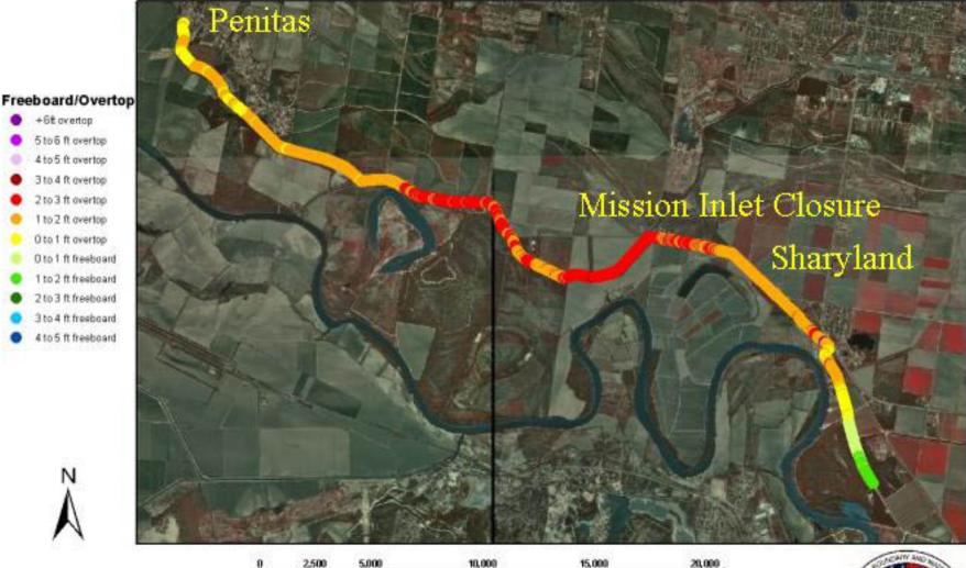
The levee within this 12 mile reach is approximately 5 feet deficient in height. Levee protects several communities from Penitas to Anzalduas Dam including the residential/industrial interests of Sharyland. Marginal geology (subsurface) concerns exist within this reach of the levee. Estimated Construction Cost - \$ 21.1 million
