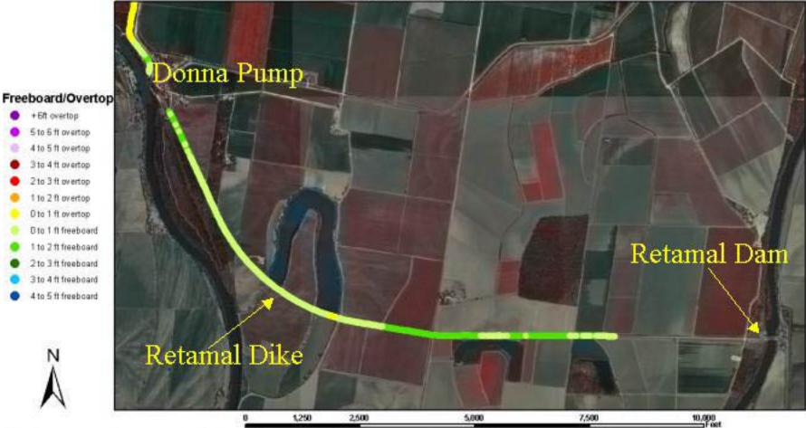
The levee reach connects Retamal Dam into the levee system and is commonly referred to as Retamal Dike. The purpose of Retamal Dam is to divert flood flows into the Mexican floodway. Failure of Retamal Dike would result in uncontrolled flows downstream of Retamal Dam. Investigations have indicated clay layers that dehydrate and hydrate; an insitu ponding test showed little seepage. Levee needs to be raised 2 feet on average. Estimated Construction Costs - \$8.8 million
