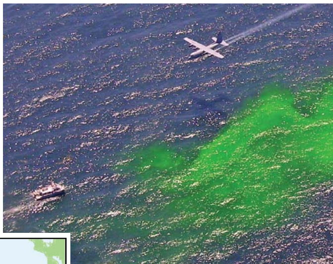
On August 9, a C-130 aircraft flown by the U.S. Air Force tests oil-spill-dispersant application by releasing water over an area of green dye representing oil spilled from the tank barge Dottie as a result of a hypothetical collision. The U.S. Coast Guard cutter Aspen, lower left, hosted elected officials and other VIPs so that they could learn about oil-spill response and see response technologies in action.
