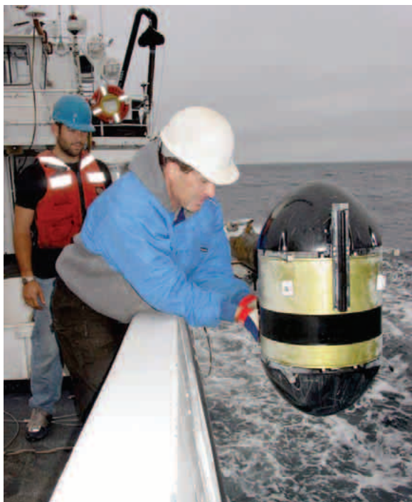
Rikk Kvitek installs the Reson 8101 multibeam-sonar head onto a rotating pipe for deployment. (The same pipe was used to deploy the ORE Trackpoint II pinger for tracking the ROV during daytime operations.) Jason Mansour assists.
