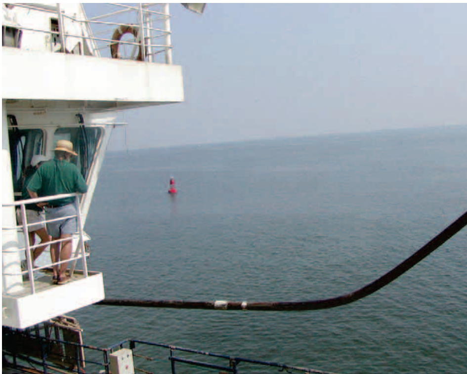
The last core recovered only 4.5 m of sediment and came up looking like a banana, as bent core pipes are called.
