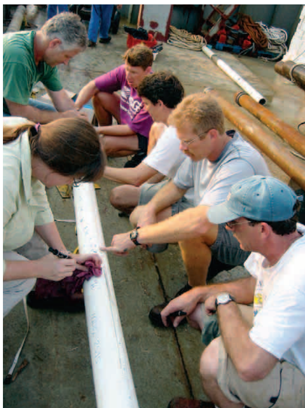
(Clockwise from bottom left) Rendy Keaten (MBARI), Charlie Paull (MBARI), Bill Waite (USGS), Jim Flocks (USGS), Tom Lorenson (USGS), and Patrick Mitts (MBARI) marking and cutting 1.5-m-long sections from one of 18 giant piston cores.
