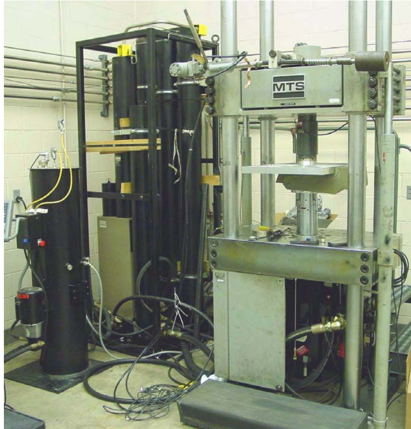
FIGURE 2-1. MTS 220-kip DYNAMIC LOAD FRAME
