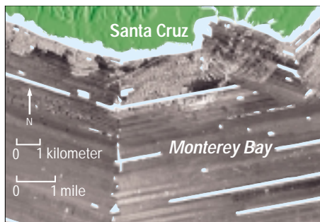
Image of sea floor off Santa Cruz, California, created from sidescan-sonar data collected in 1995 and 1996. Parallel bands in broad V-shape are swaths of sidescan-sonar data. Dark areas are muddy sediment. Bright areas are outcrops of bedrock and patches of sand. Light line angling southwestward from Santa Cruz is an outfall pipe.
