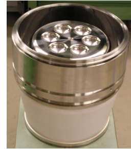
Figure 2: Electron Gun of the E3736
