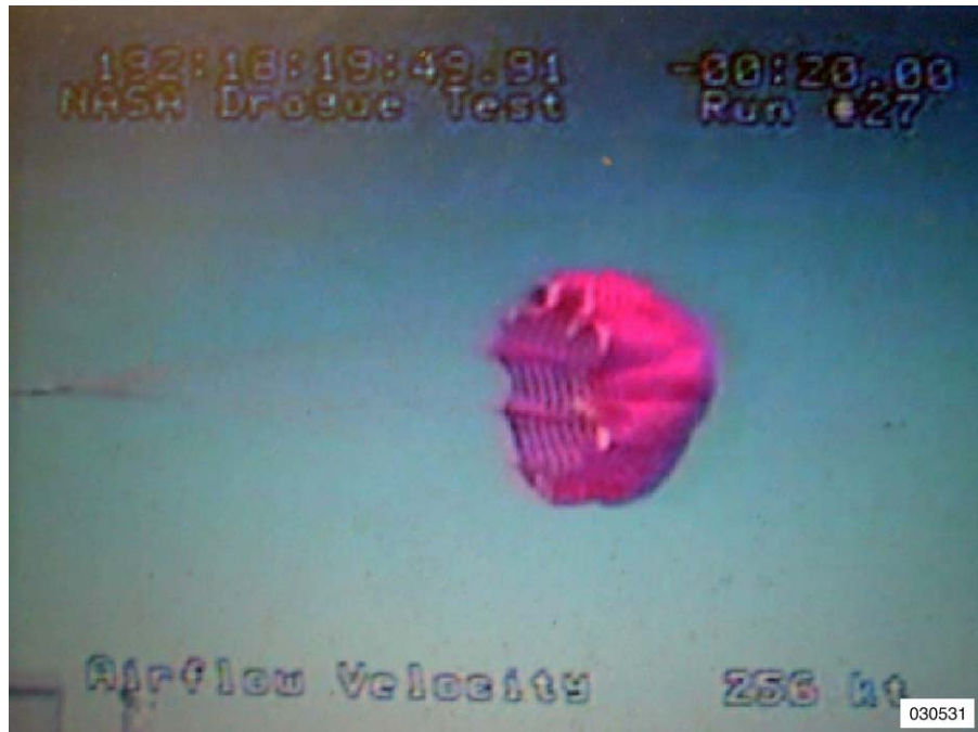
(a) Original 24-percent ribbon drogue parachute design.
