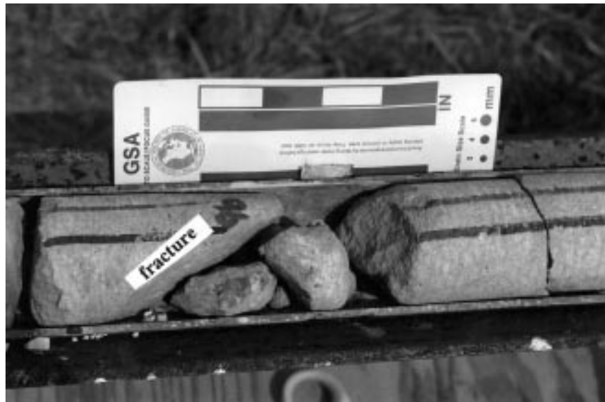
FIG. 8. Natural fracture in GW-6 core between 24.9 m and 25.1 m depth. The top of the core section is on the left. The core piece on the left has a planar, natural fracture surface oriented 30° to the core axis. The other side of the fracture has been broken into rubble because of coring. The scale is 10.16 cm (4 inches).
