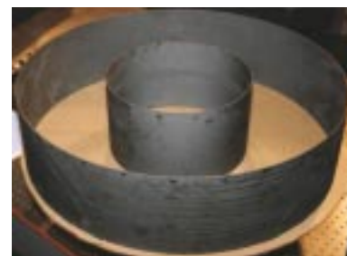
Fig. 4. Photograph of 30-in. diam/13-in diam MI SiC/SiC combustor liner pair used in an advanced turbine.
