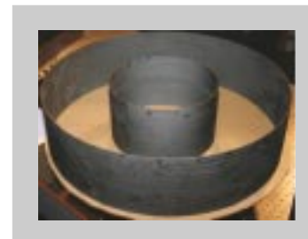
Fig. 4. Photograph of 30-in. diam/13-in diam MI SiC/SiC combustor liner pair used in an advanced turbine.
