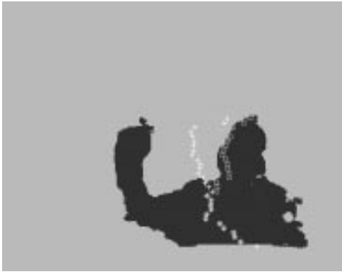
Fig. 4. Illustration of the horizontal mean values (pluses) vs. horizontal median values (squares). Notice how much more the means are affected by the waving arm.
