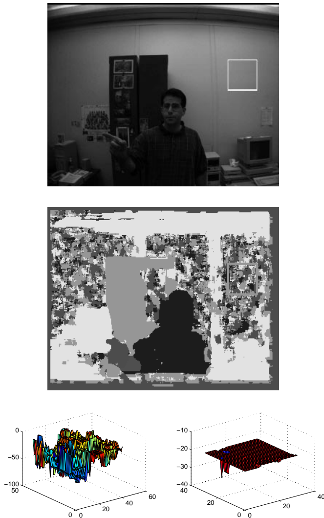
Fig. 1. TOP: Sample input image from camera. White square highlights region with little texture. MIDDLE: Disparity image from the Digiclops TM Stereo System from Point Grey Research, Inc. Note noise in the highlighted region. BOTTOM LEFT: Reconstruction of physical surface based on disparity values in highlighted region (negative z axis trends away from camera). BOTTOM RIGHT: Reconstruction of physical surface based on region centered inside of the human figure in the middle.
