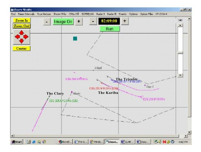
This diagram, taken from appellee the Clary's brief and intended only as a guide to aide the reader's visualization of the events surrounding the collision, illustrates the positions of the three vessels at approximately 2:09 on December 4, 2002. The dashed lines represent the bounds of the Traffic Separation Scheme. The arrows represent the vessels and their directions.
