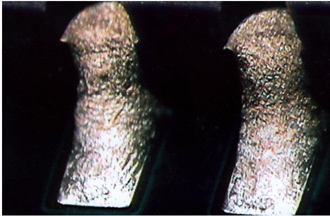
SACB termination soldered with SnPb
