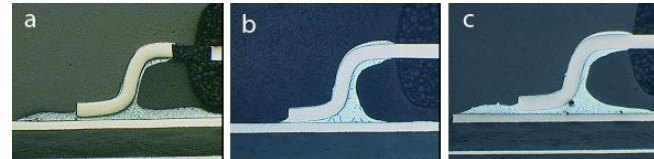
Sn TQFP-144 reflowed with (a) SnPb, (b) SAC and (c) SACB
