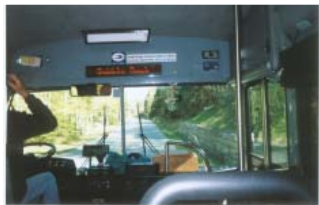
Figure 4-5: Automatic Annunciator Text Display On-board the Island Explorer Bus 21
