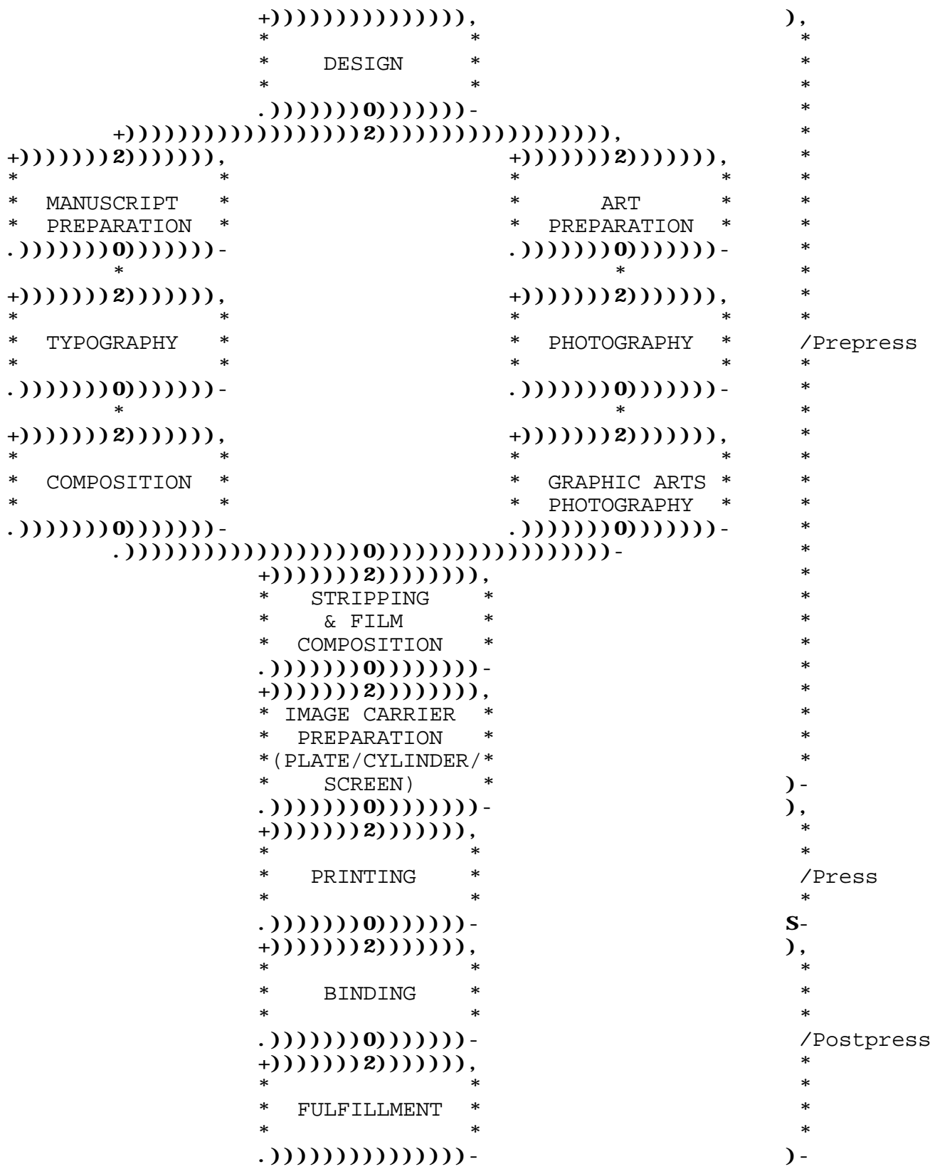
Figure 9. Flow Chart of a Typical Printing Process (Source: Field 1980).
