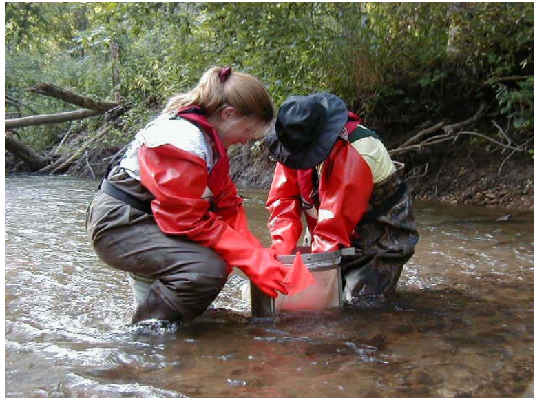
Figure 1. Using modified Hess sampler in stream riffle. Photo by Sarah Tegt, USGS, July 2000.
