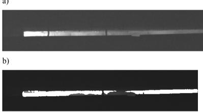
Fig. 8: Fire according to test-case 3 (smouldering wood fire, t = 400 s after start of the experiment), seen through the gap between the container's top edge and the ceiling.
