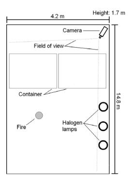
Fig. 1: Cargo bay mock-up (Airbus A340) as used within the framework of the fire tests
