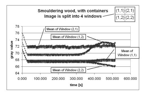
Fig. 7: Time-dependent mean for a smouldering wood fire, with containers (Test case
