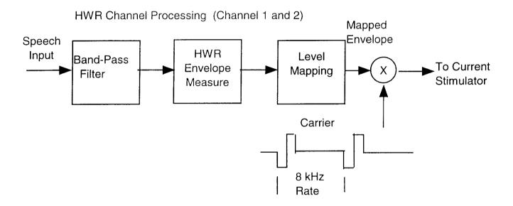
Pulsatile Timing Sequence (Channels 1 and 2 @ 8 kHz, 3-6 @ 4 kHz)
