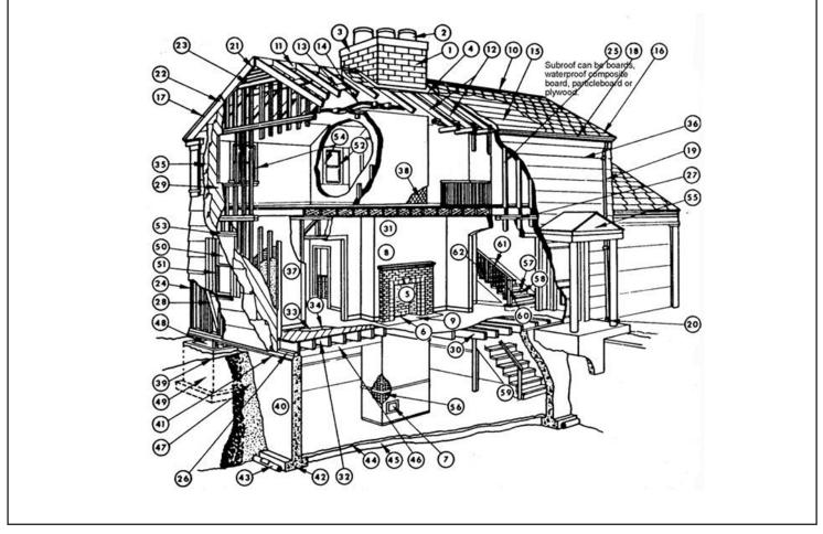
Figure 6.2. Housing Structure and Terminology, Typical House Built Between 1950 and 1980 [2]
