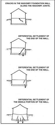
Figure 6.4. Foundation Cracks [4]
