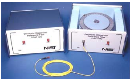
Figure 15. SRM 2524, Chromatic Dispersion Standard.
