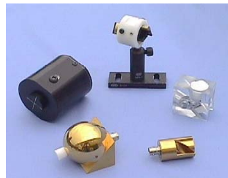
Figure 13. Several light-trap detectors—transfer standards designed to collect and absorb virtually all of the light incident upon them.
