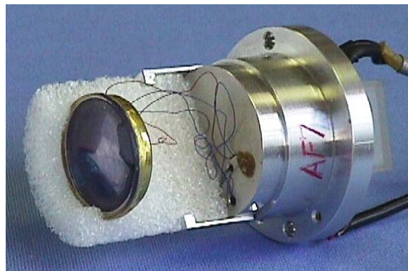
Figure 1. Liquid cell calorimeter; first primary standard for laser measurements developed at NBS.
