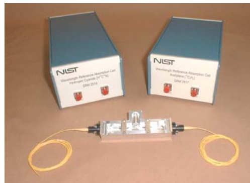
Figure 18. SRMs for wavelength calibration: absorption cell in front and packaged units in back
