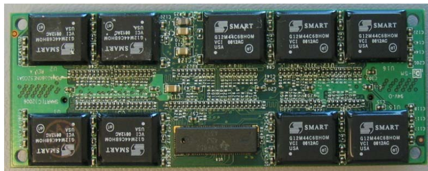
Figure 15: Top Side of 4 GB Memory Module
