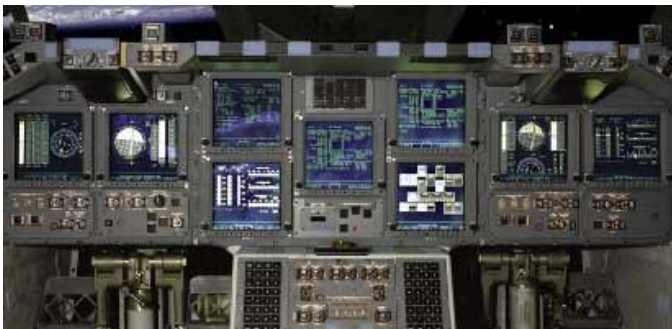
Figure 1. Nine MDUs in the forward flight deck of MEDS cockpit (NASA photo)
