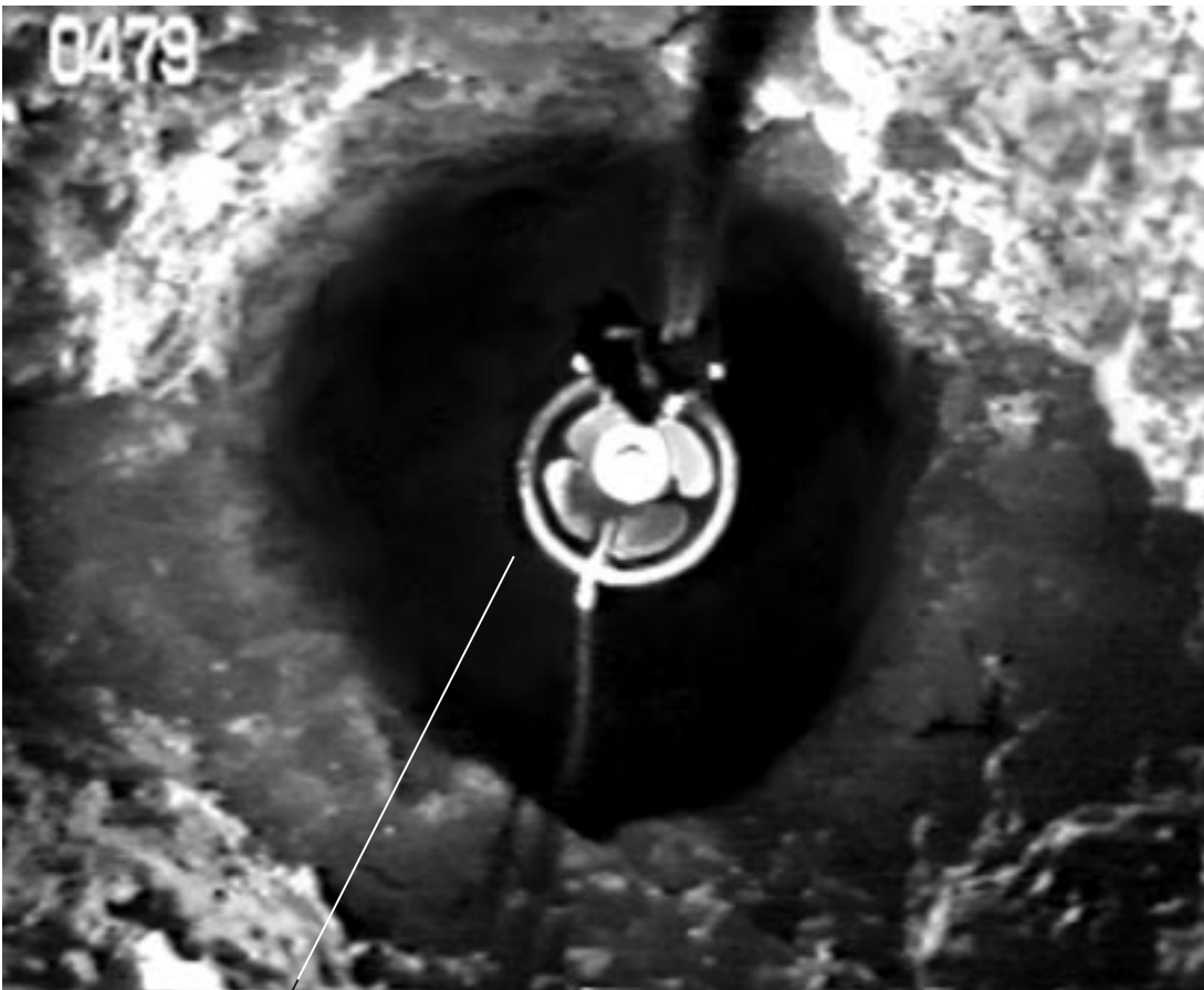
Figure 7. A borehole video camera with the impeller flowmeter attachment in a 12-inch open borehole at a depth of 479 feet below land surface.
