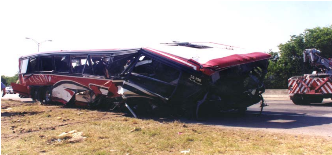
Figure 5. Body damage to bus, which had been moved from its resting position when this photograph was taken (photograph by the New Orleans Police Department).
