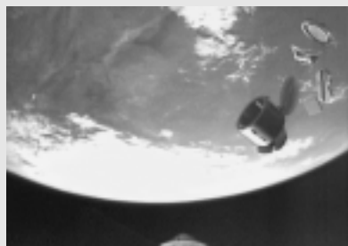
Video frame shows experiments ejecting from sounding rocket. The first ejection was the scramjet flight dynamics experiment.
