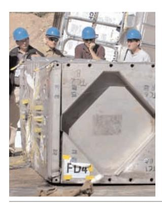
Sandia's Aerial Cable Site has been busy in recent weeks, conducting a number of tests, including this drop test of a TRUPACT-III container. Constructed by Packaging Technology, or PacTec, for Carlsbad-based Washington TRU-Solutions, the TRUPACT-III is based on a French design adapted by the company. The container tested is a one-half scale model of the actual container, which would be used for contact-handled transuranic wastes too large for the original TRU-PACT-II containers.
