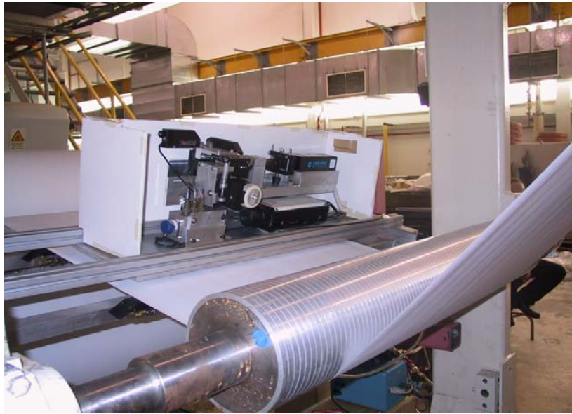
Figure 3. LUS system installed on pilot coating machine.
