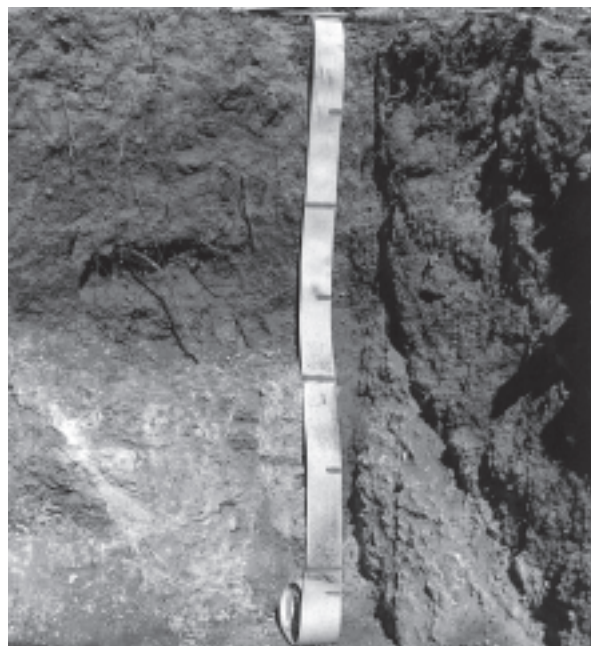
Figure 14.—Profile of Freshwater stony loam in an area of Roca-Freshwater stony loams, 2 to 20 percent slopes. A duripan is at a depth of about 18 inches and is underlain by bedrock.
