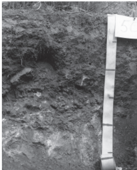
Figure 16.—Profile of Roca stony loam in an area of Roca-Freshwater stony loams, 2 to 20 percent slopes. Fractured bedrock is at a depth of about 22 inches.
