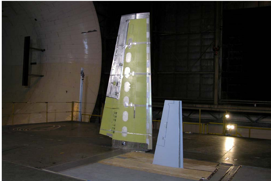
(a) Full-scale and 5/12-scale models in LFST test section.
