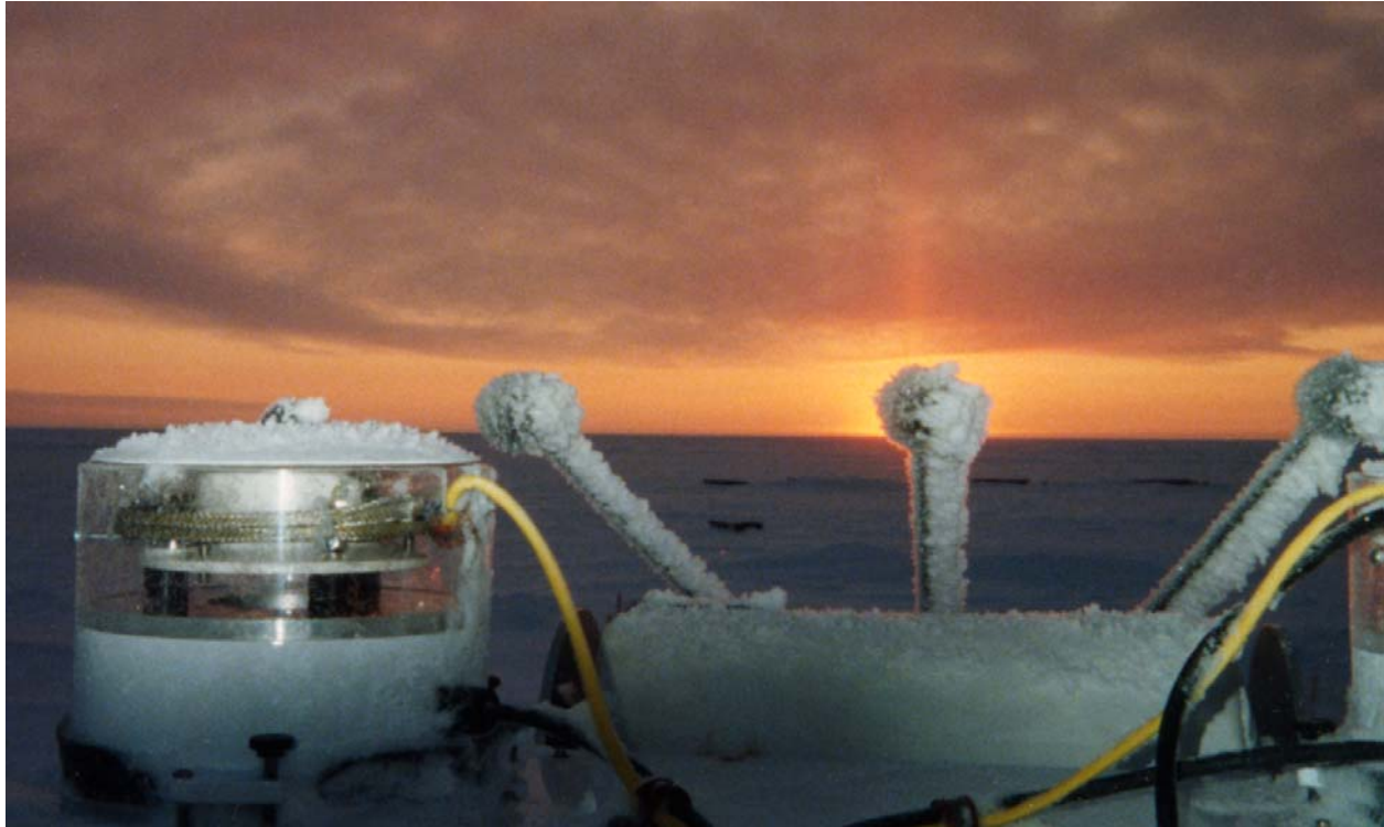
Figure 5.10. Hoarfrost on ARM/SHEBA Instrumentation
