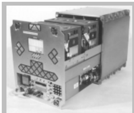
The Biomass Production System (BPS) is an engineering development unit for a future International Space Station (ISS) plant habitat capable of supporting long-term plant growth and botanical experimentation in space.
