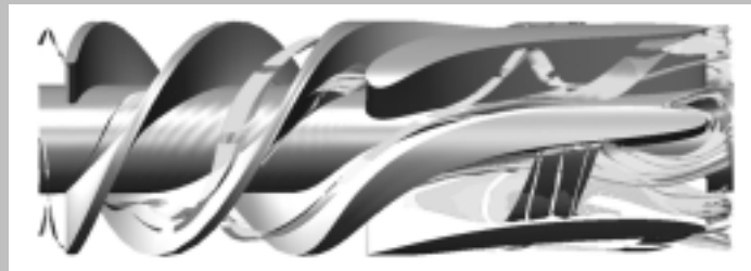
Particle traces shown inside the inducer-impeller section of Ventricular Assist Device (VAD).
