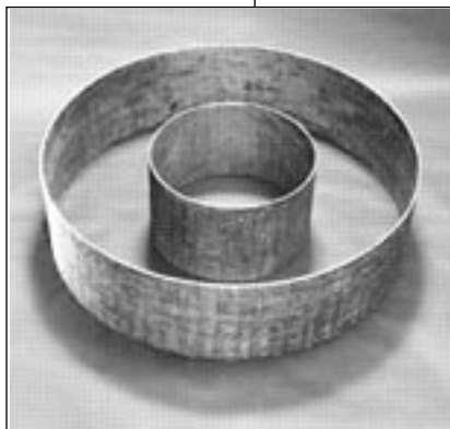
Fig. 2. Full scale 3D woven SiC/SiC liners fabricated by B.F. Goodrich Supertemp.
